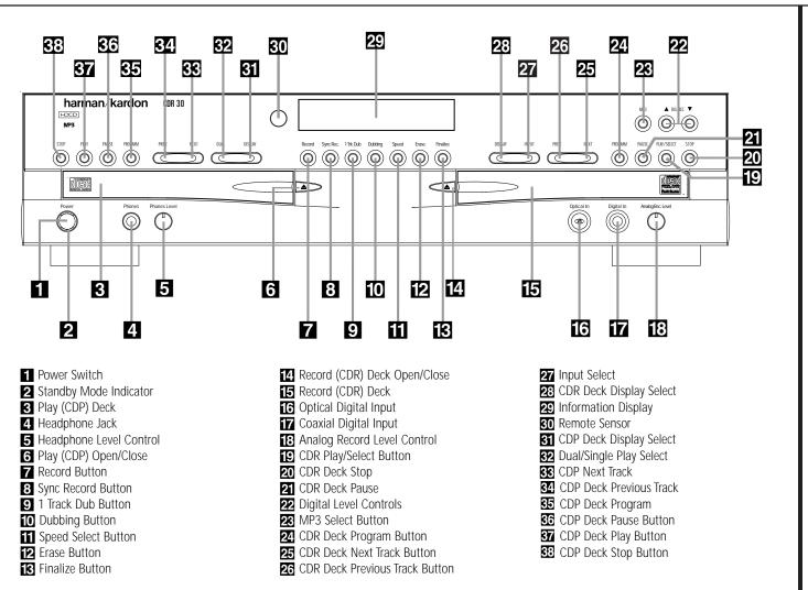
Dower Switch: Press this switch to apply power to the CDR 30. When the unit is first turned on, the **Standby Mode Indicator** 2 surrounding the switch will turn green. Once the unit has been turned on with this switch, it may be operated from either the front panel or remote control. Press the switch again to turn the unit completely off.
